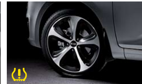
TPMS The tire pressure monitoring system constantly monitors all four tires and alerts the driver via a warning light on the instrument cluster if any tire's pressure drops below the safe range.
