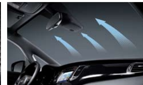
Auto defogging system A sensor automatically initiates a defogging process when condensation is detected on the windows to ensure optimal visibility in humid climates.
